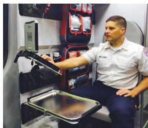
Pulaski County requested a forward-facing seat instead of the typical side bench seating for more safety and better access to the patient and medical supplies.
