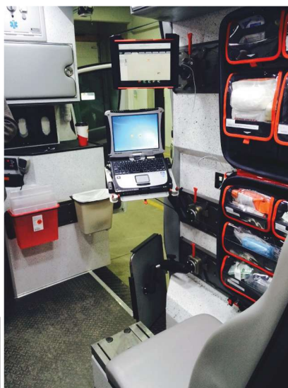
Several soft-sided supply bags and monitors are easily moved around the ambulance on the tracks, based on the needs of each call.
